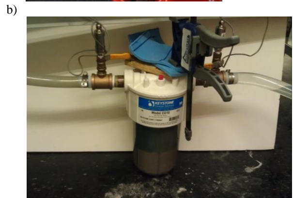
FIGURE 6: a) Experimental drip irrigation setup. b) Experimental filter assembly with dual pressure transducers. Unfiltered water flowed from the left, and the pressure transducers measure pressure before and after the filter.
