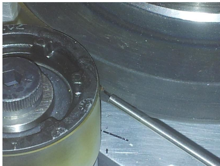
Figure 15: A picture showing how a fiber is held against the black capstan by a silicone conveyor band.
