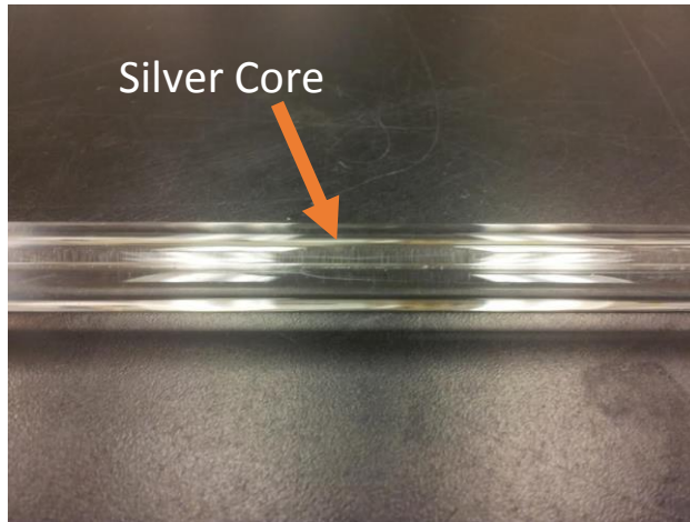
Figure 2: A preform with Silver as the core and silica as the cladding.
