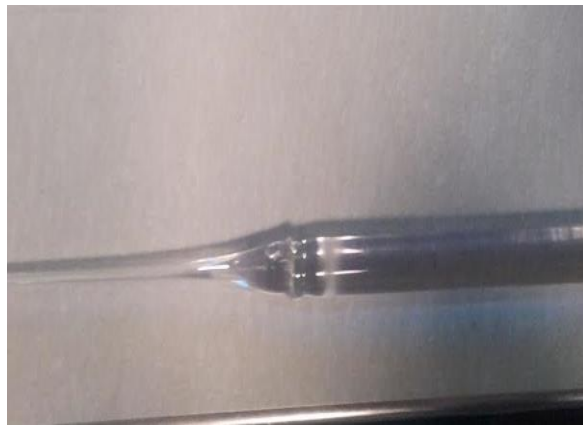
Figure 1: (a) Various post-draw preforms made with a thermoplastic cladding. Figure courtesy of Greg Hren. (b) Post-draw preform made with a glass cladding. Both preforms exhibit the bulk, beginning preform at the bottom and a scaled down portion at the top.
