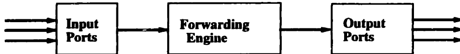
Figure 5-1: The functional description of a router is composed of Input, Forwarding and Output modules.
