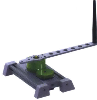
Figure 4-6: LTEye Sniffer Prototype. Prototype of the rotating antenna on a LTEye sniffer.
