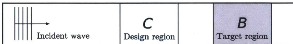
Figure 5.1: Frequency filter geometry in 1d. C is the pixelized design region and B is the objective subdomain.
