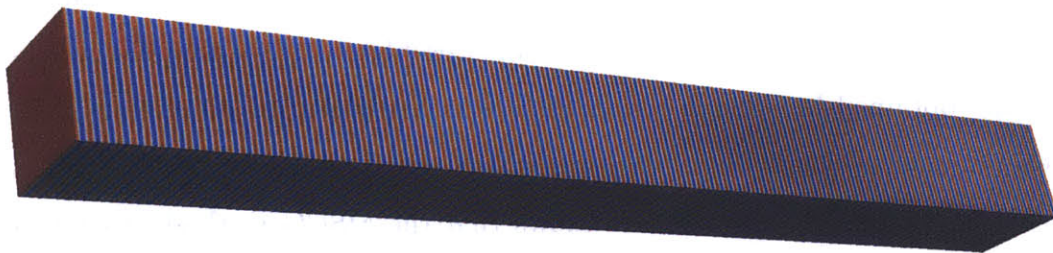
Figure 2.13: Acoustic wave propagation pattern for a 3d homogeneous rectangular prism. The domain size is 10 \times 10 \times 100 wavelengths.
