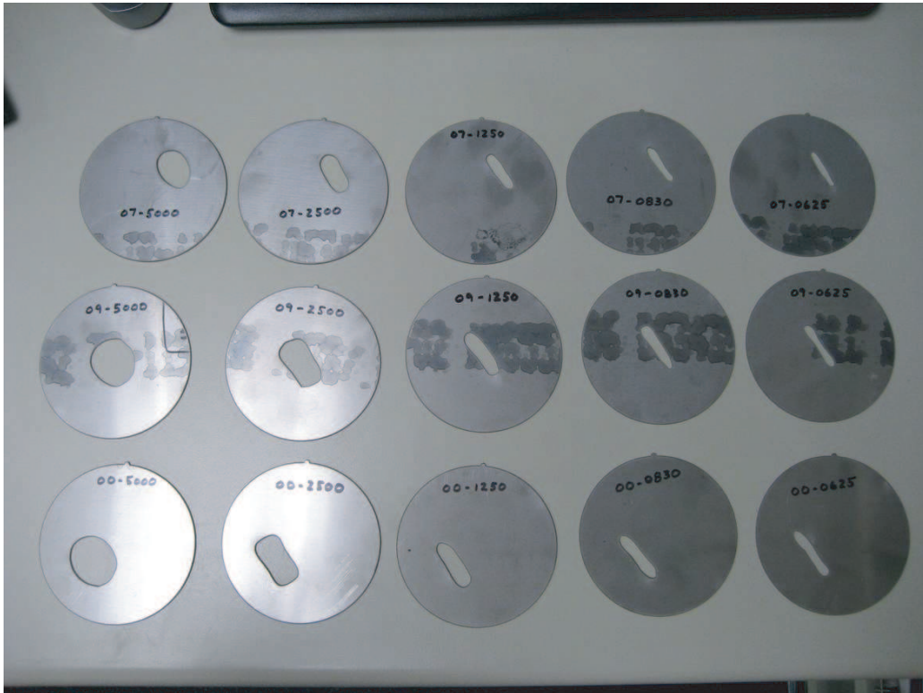
Figure B-6: Aperture plates fabricated based on the images shown in Fig B-5 (b) and used to mimic the L1 aperture shown in Fig B-5 (a) during the FY2007 campaign.
