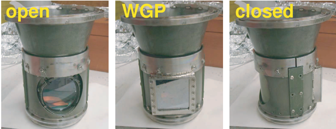
Figure 2-6: Three possible rotational positions of the upgraded MSE shutter. The WGP allows the MSE system to respond to non-motional-Stark-effect-induced polarized light. The shutter is controlled by the push-pull mechanism.
