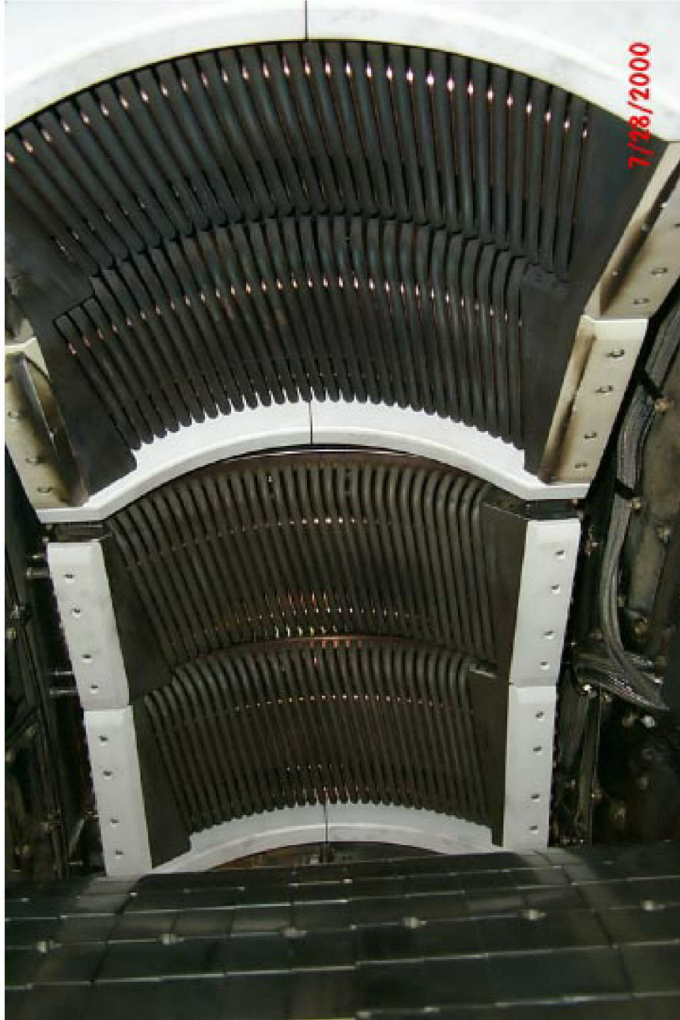
Figure 1-4: A view of the D- and E-port antennas from inside Alcator C-Mod. (Turn the page clockwise 90° to view correctly).
