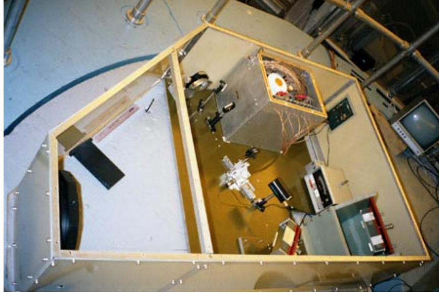
Figure 2-22: PCI imaging optics and detector array on top of the Alcator C-Mod igloo
