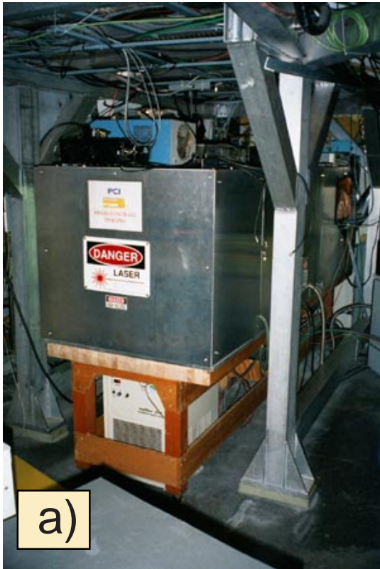
Figure 2-19: The optical table housing the CO 2 laser and the beam expansion optics.
