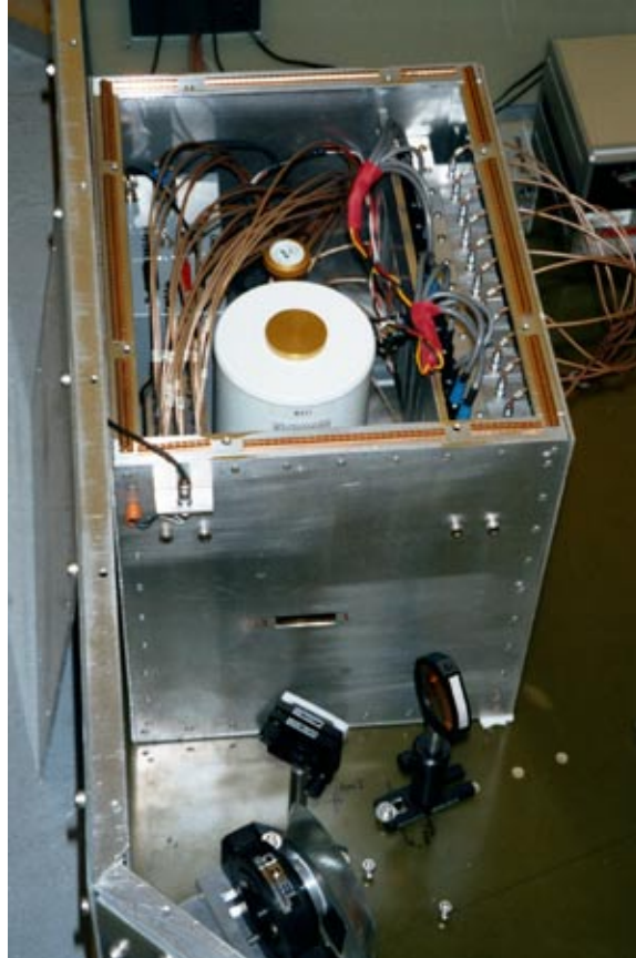
Figure 2-24: Shielded box for the detector array, the preamplifiers and the battery power supply.
