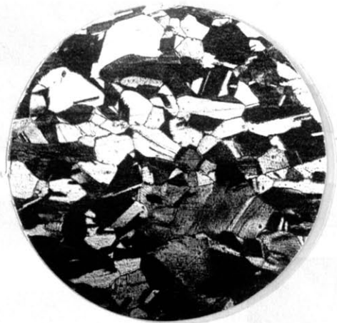
Figure #12. Original Alpha Brass, as received. 125 X.
