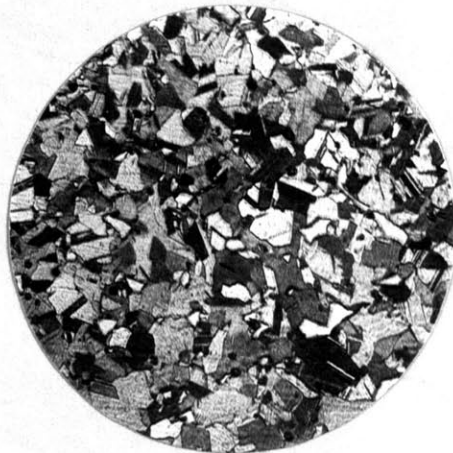
Figure #4. Muntz Metal - M-800-1/4. .120 in. cup. Heated 800° F.- 30 mins. 125 X.
