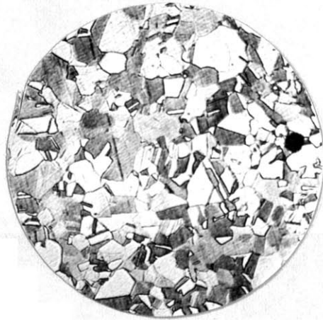
Figure #15. Alpha Brass - A-1010-1/2. .180 in. cup. Heated 1010° F. - 30 mins. 125 X.
