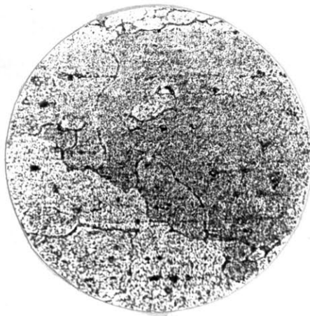
Figure #26. "Al." Alloy - 17 ST-925-3/4. .190 in. cup. Heated 925° F.- 60 mins. 200 X.
