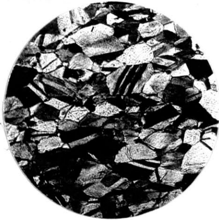
Figure #2. Muntz Metal - Full worked. .450 in. cup 125 X
