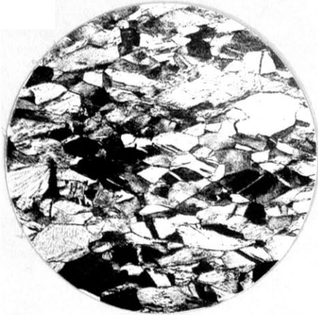
Figure #13. Alpha Brass - Full Worked. .345 in. cup. 125 X.
