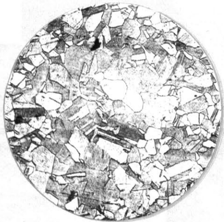
Figure #16. Alpha Brass - A-1010-3/4. .270 in. cup. Heated 1010° F. - 30 mins. 125 X.
