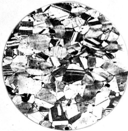
Figure #3. Muntz Metal - M-620-3/4. .360 in. cup. Heated 620° F.- 30 mins. 125 X.
