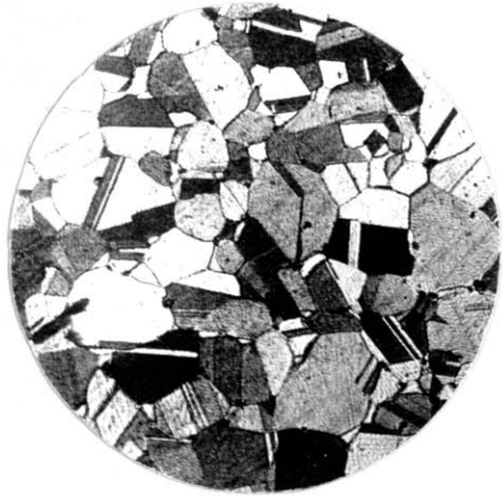
Figure #1 Original Muntz Metal as received. 125 X
