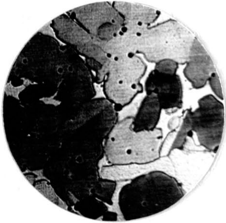
Figure #9. Muntz Metal - M-1550-1/2. .235 in. cup. Heated 1550° F. - 30 mins. 125 X.
