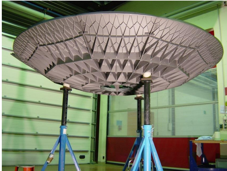
Figure 20: The Herschel telescope primary mirror with ribbed backstructure 23
