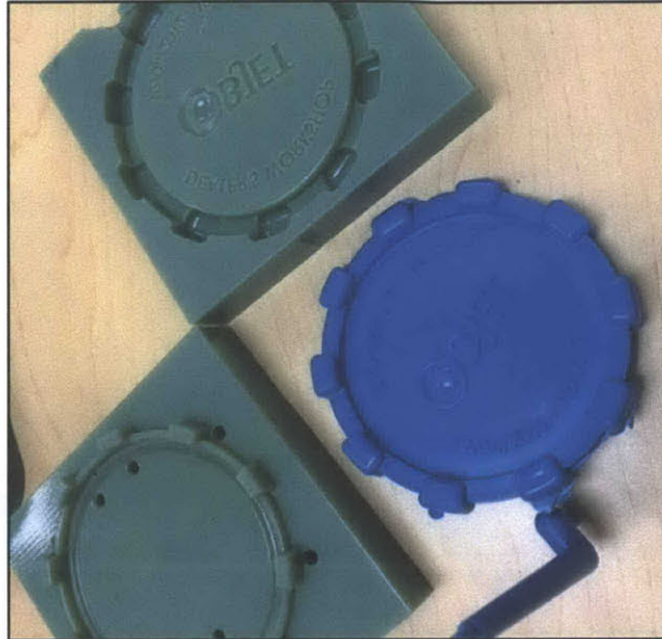
Figure 10: 3D printed mold used in an injection molding application
