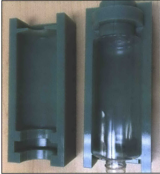
Figure 9: 3D printed mold used in a blow molding application
