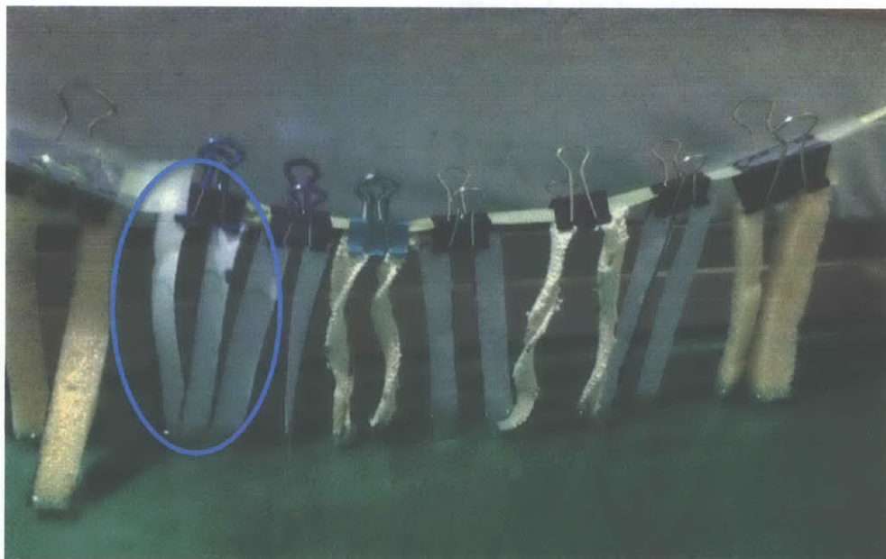
Figure 12: Results of vertical wicking test after 2.5 hours. Only cotton cloth exhibits signs of significant wicking.
