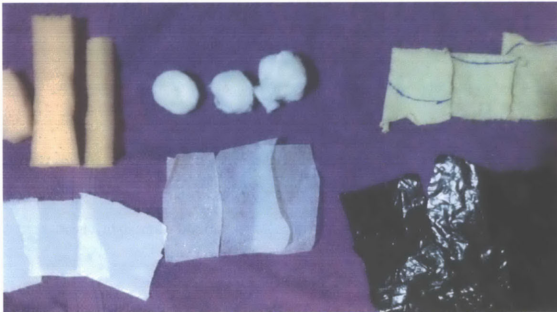
Figure 2: Raw materials used for testing. From left to right by row: foam, cotton balls, mutton cloth, cotton cloth, interfacing/stiffener, and plastic
