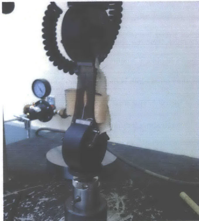
Figure 13: Strain of Mix 1 (plastic, foam, mutton cloth) in Instron. Fracture of the plastic is evident before other materials.
