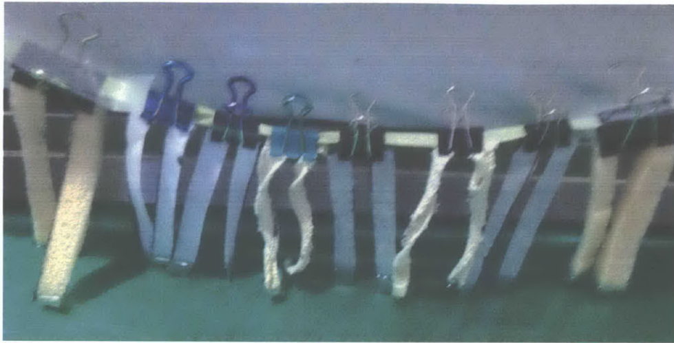
Figure 11: Setup for vertical wicking, four samples for each material. From left to right (two samples per clip): Foam, cotton cloth, mutton cloth, interfacing, mutton cloth, interfacing, foam)
