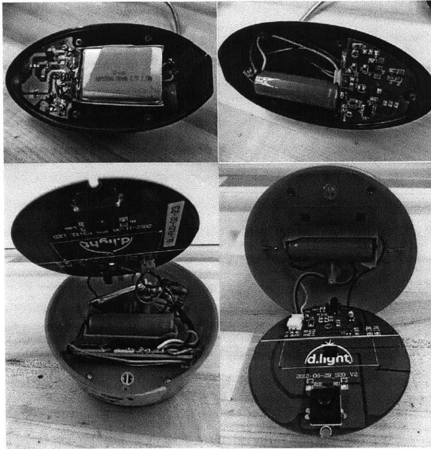
Figure 30: Solar Lanterns with Instrumentation Embedded. Left: Instrumented Lanterns. Right: Normal Lanterns.
