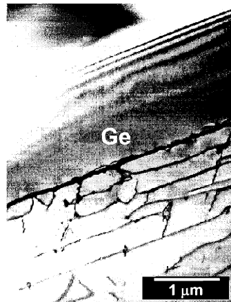
Figure 3.10 Cross-sectional TEM micrograph of the uniform Ge cap and upper graded buffer layers of sample D.
