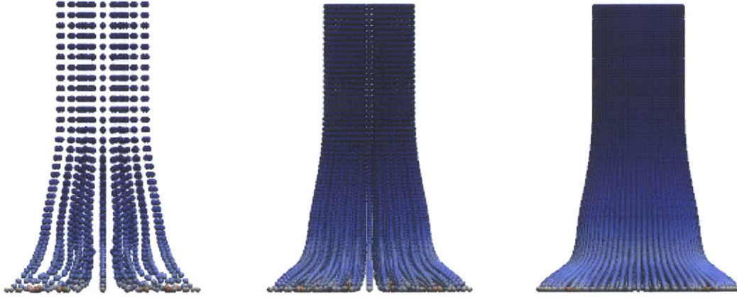
Figure 3-1: Simulated final configurations of a Taylor impact test for discretizations D1 (left), D2 (center), and D3 (right).
