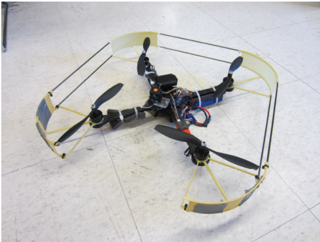
Figure 1. AscTec quadrotor equipped with onboard camera and GPS receiver
