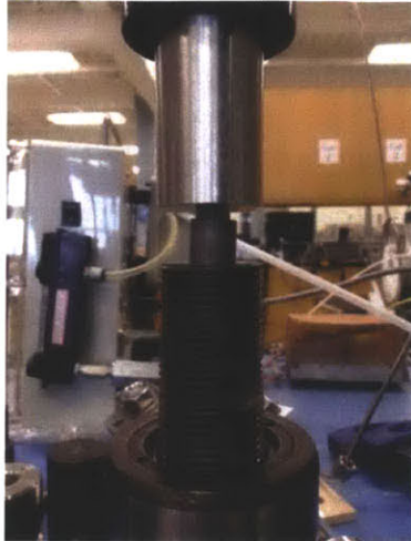
Figure 2-35 Picture of the Burst Experiment Facility when Loaded with a SiC Sample
