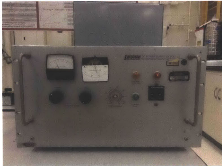
A3: Power Supplier of the Sample Furnace of the Oxidation Facility
