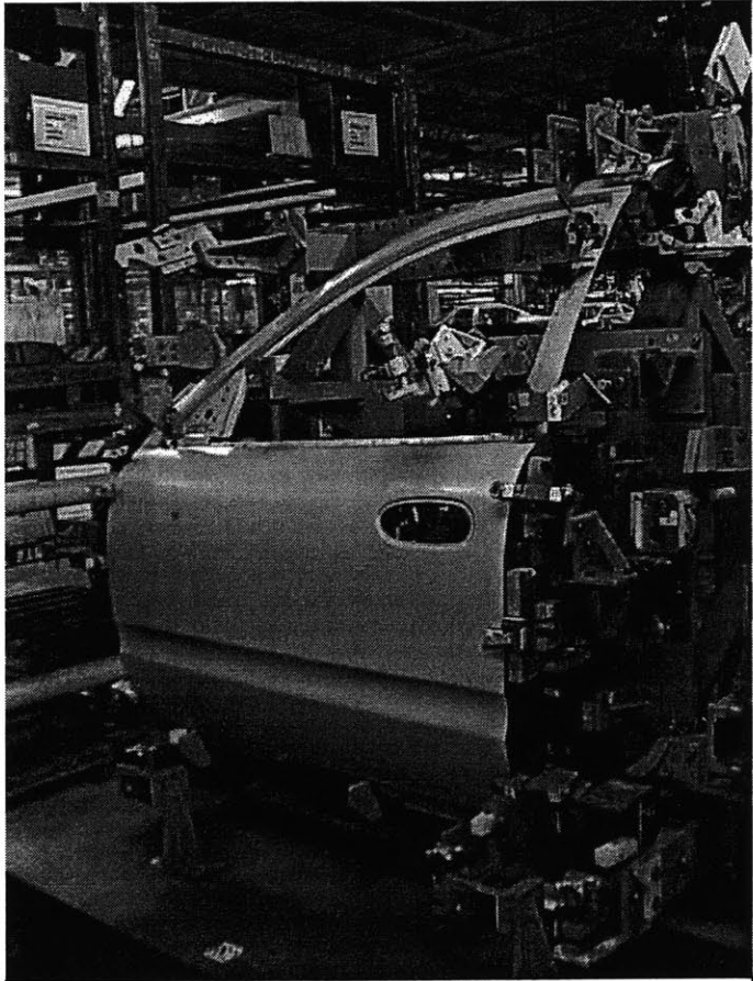
Figure 3.10: Hinge Placement Check Fixture
