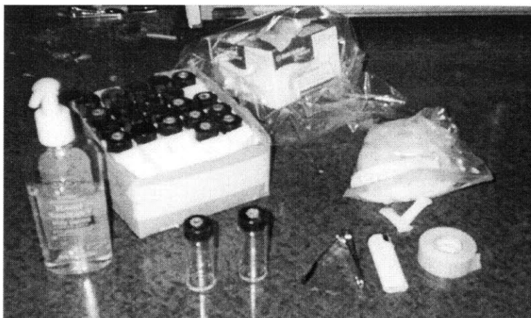
Figure 4.9 H 2 S test field equipment: hand sanitizer (left) with 20 mL sterilized glass vials, nail clippers, lighter, marking tape and powdered media capsules.
