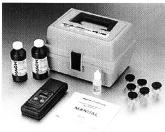
Figure 4.10 Turbidimeter field kit. Counter-clockwise from left: calibration standards, pocket turbidimeter, instruction manual and sample vials (HACH, 2003).
