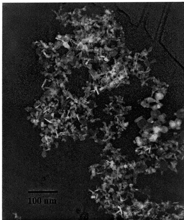
Figure 4-8. TEM micrograph of nanocrystalline AlN produced at 7 mbar in a 2.3-slp m gas stream with 27 vol% NH 3 and 73 vol% He.
