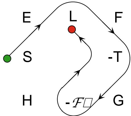
$$(-1) \left( \frac{\partial S}{\partial L} \right)_T = \left( \frac{\partial \mathcal{F}}{\partial T} \right)_L = b(L - L_0)$$
