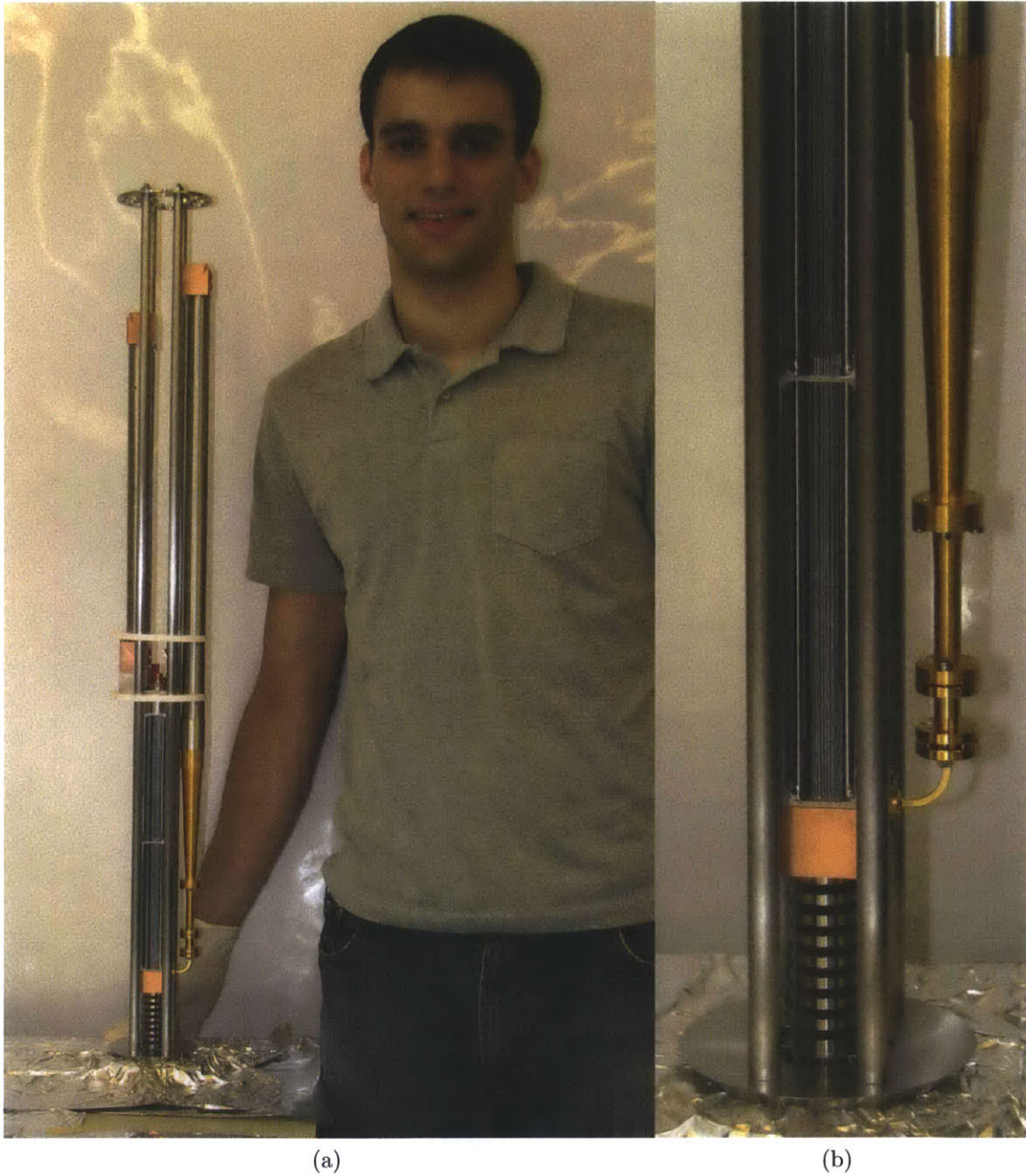
Figure 6-10: (a) Fully assembled amplifier insert with the input corrugated waveguide on the right and the output on the left. (b) Close-up of the corrugated horn mated to the wraparound coupler and PBG circuit which is supported by the final section of the slotted beam tunnel. Venting holes for the first section of the beam tunnel and the electron gun are visible on the mounting plate (bottom) around the slotted beam tunnel.
