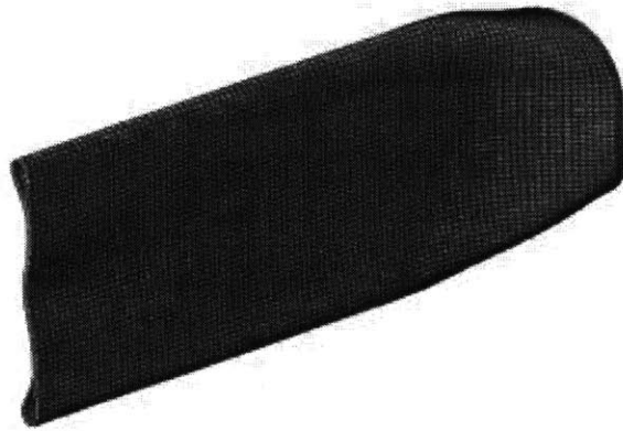
(a) Symmetric collapse (charge size=100 g TNT).
