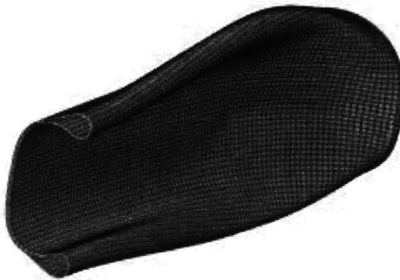
(b) Asymmetric collapse (charge size=500 g TNT).
