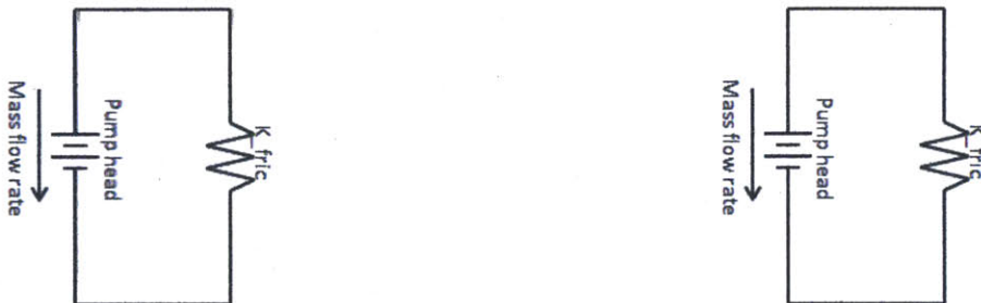
Figure 75: Network reduced to a single pump and a single equivalent resistance to flow per isolated loop
