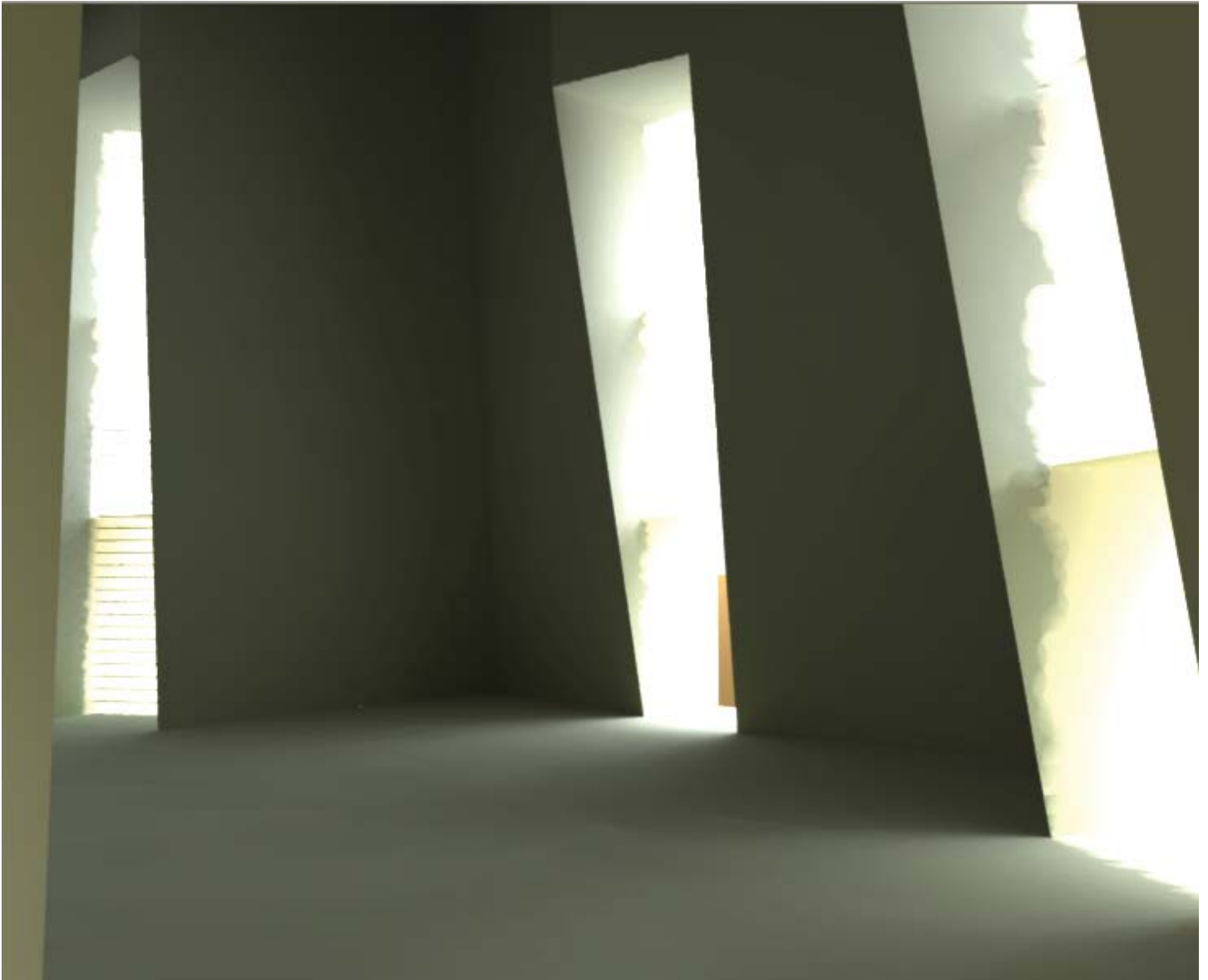
Radiance: Simulation of Daylighting Effect CIE Overcast Sky 6 Indirect Reflections Quality: High
