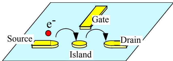
The above figure demonstrates the idea of CNT single electron transistor by AFM nicking. The nanotube is broken at two locations and electrons will transfer from source to drain under specified applied tip voltage.
