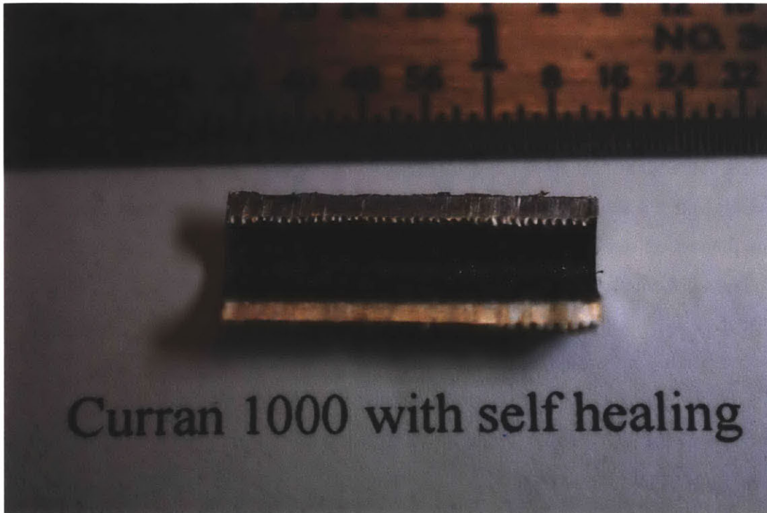
Figure 68-Deposition on the Curran 1000 with self healing tested during Test 4. Tick marks are 1/64th of an inch.
