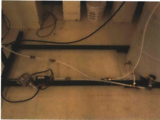
Figure 35 - The pump can be seen below along with the bypass back to the reservoir.
