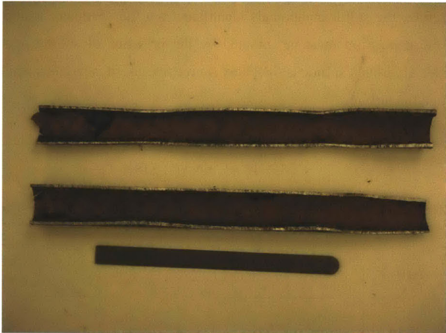
Figure 7-The 10" section of the sample DCT fouled pipe.
