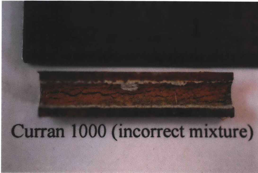
Figure 60-Deposition on the Curran 1000 sample tested during Test 2. Tick marks are 1/64th of an inch.
