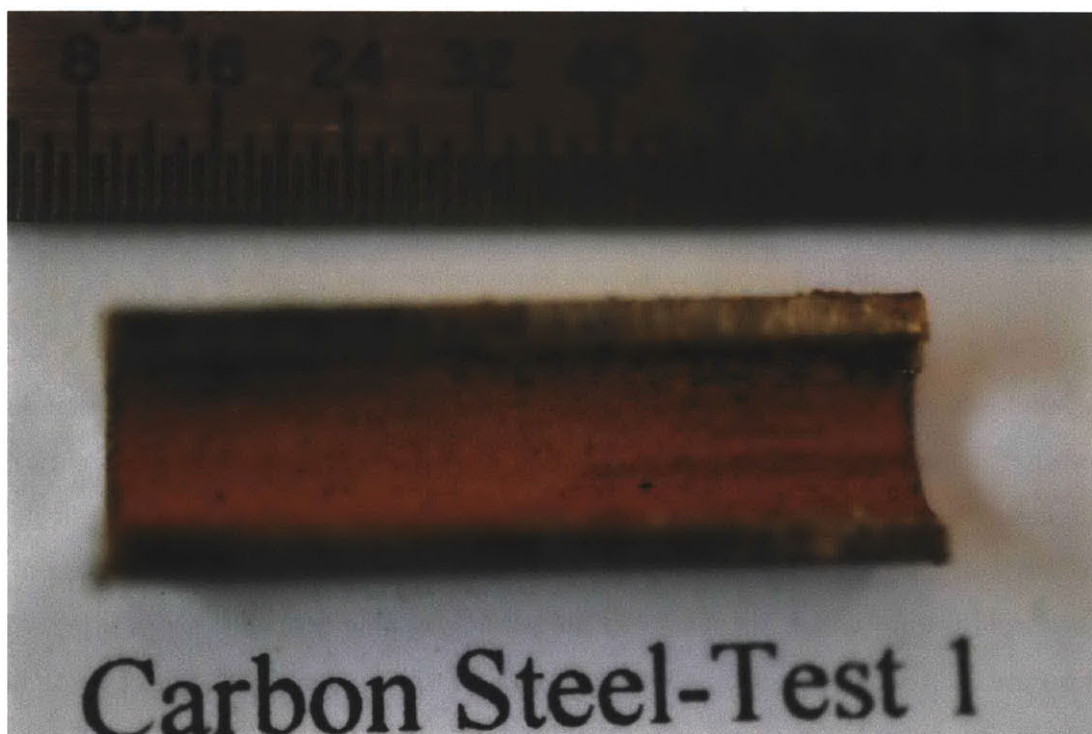
Figure 55-Deposition on the carbon steel sample tested during Test 1. Tick marks are 1/64^{\text{th}} of an inch.
