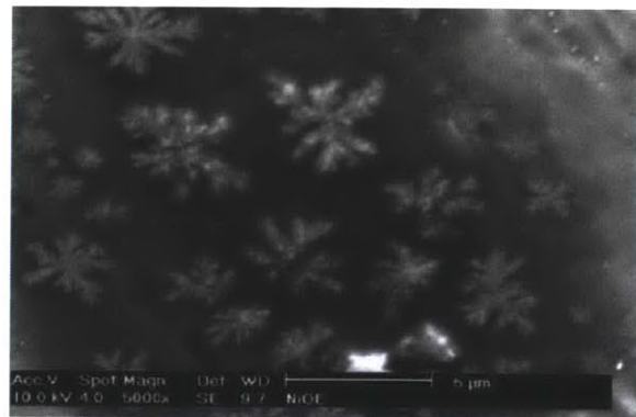
Figure 17-A dendrite structure created by amorphous nanoparticles embedded in NiO (Katumba, Olumekor and Forbes).
