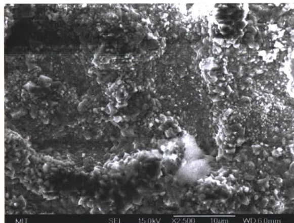
Figure 42-Structure of the surface of the 617 samples obtained with the SEM.
