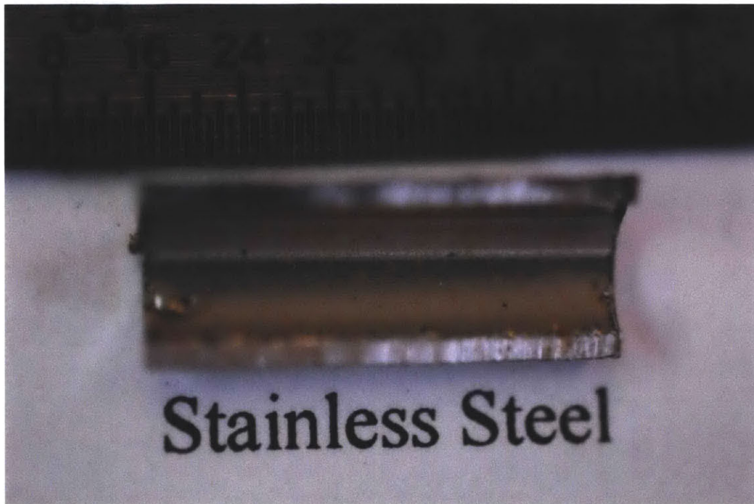
Figure 56-Deposition on the stainless steel sample tested during Test 1. Tick marks are 1/64th of an inch.
