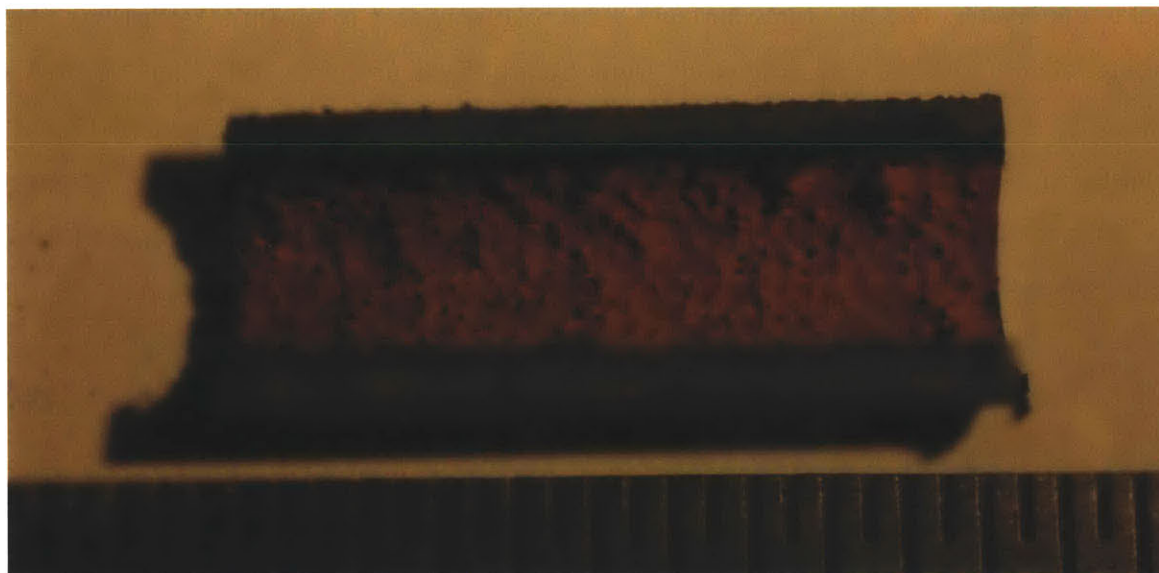
Figure 39 - View of the deposition on the carbon steel samples from the validation trial from the sectioned sample. Tick marks are 1/64 th of an inch.
