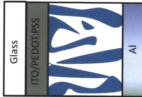
Figure 3.7 This illustration only shows the physical structure of the device, the energy levels are not indicated. Typical anode and cathode are shown the structure. The blue and white swaths in the active layer are representative of the donor and acceptor materials.
