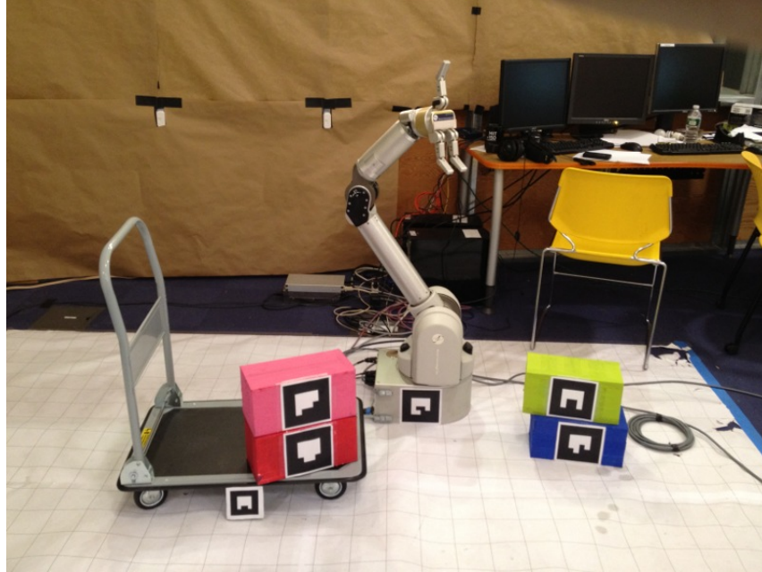
Figure 4-1: Our implementation of a robotic manufacturing agent. The Barrett WAM (Whole Arm Manipulator) is capable of manipulating colored blocks, which are each marked with a fiducial for sensing purposes. It is capable of robustly creating assembling stacks of blocks on the cart.
