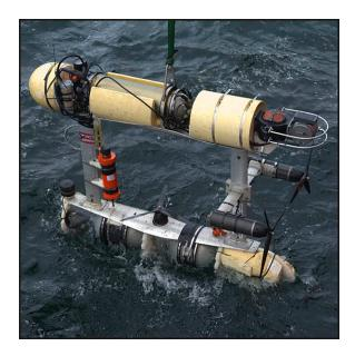
Figure 1-1: The Seabed AUV without its fairings, in under ice configuration. The upper hull contains the control computer, multibeam sonar, doppler velocity log, and camera. The lower hull contains batteries and the fibre optic gyro. Additional science sensors are scattered around the robot. An ultra-short baseline transponder is mounted to the front strut.
