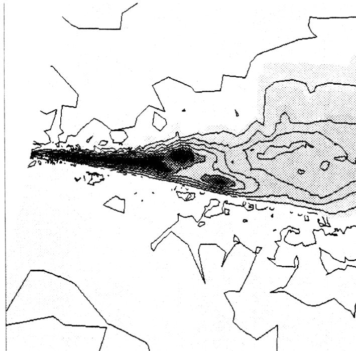
Figure 4.33: Computed variation of axial velocity through the vortex core, for \alpha = 42^\circ , on coarse mesh. Contour increment is 0.1, innermost contour value is 0.
