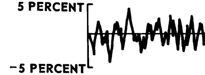
Fig. 2-8. Hovering performance of velocity control system under gust conditions (30 fps peak gusts).
