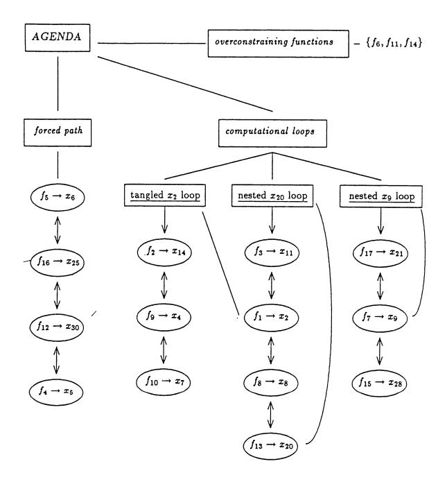
Figure 2.3: A computational agenda structure with nested and tangled loops.
