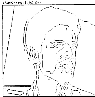
Walter and Canny's edges with \sigma = 1.63 and \sigma = 1.57 . Cross-validation: \sigma = 1.57 pixels, standard-regularization: \sigma = 1.62 pixels. We solved equation 5.b since So/No ratio smaller than 200.
