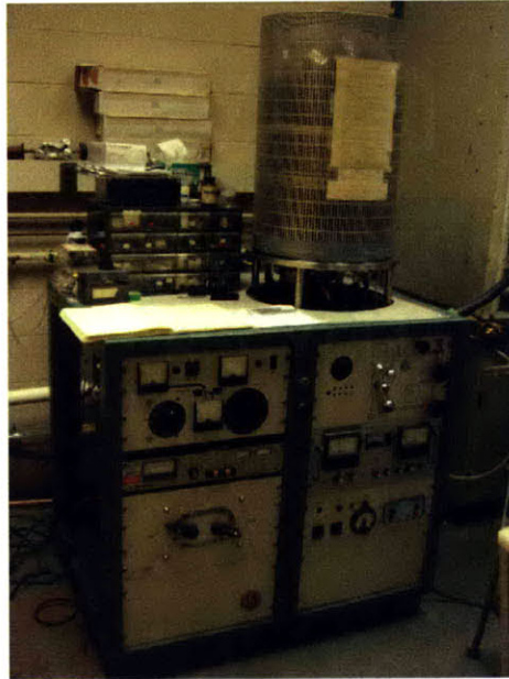
Figure 3-7: Fonstad thermal evaporator in room 13-3024.
