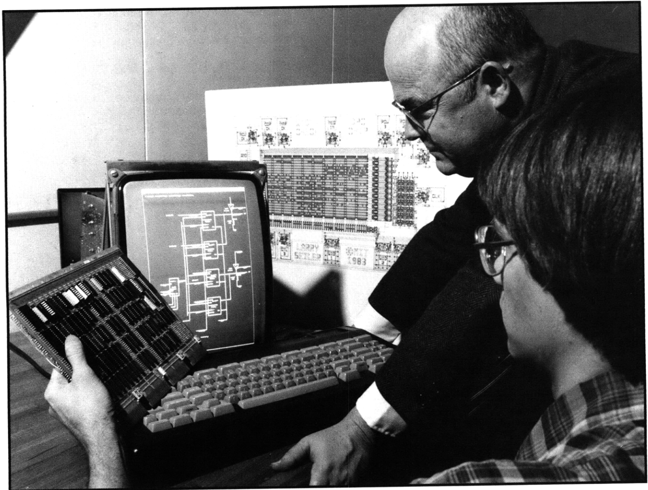
From left, Professor Jonathan Allen, Director of the Research Laboratory of Electronics, and graduate student Larry D. Seiler are inspecting the design of a system for high-speed design rule checking which uses four custom integrated circuits in a novel architecture.
