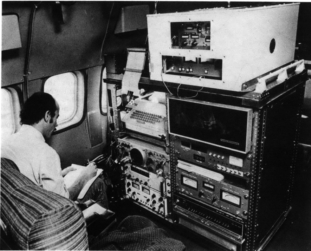
Fig. I-8. 53-GHz radiometer-spectrometer system in operation on the NASA Convair 990 aircraft.
