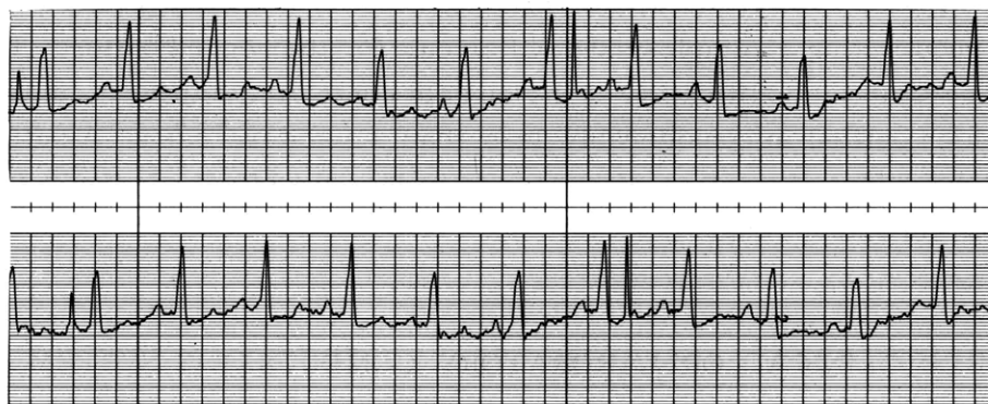
Fig. XIII-4. Example of signal delayed 500 ms. Upper channel: undelayed original. Lower channel: delayed, quantized output.
