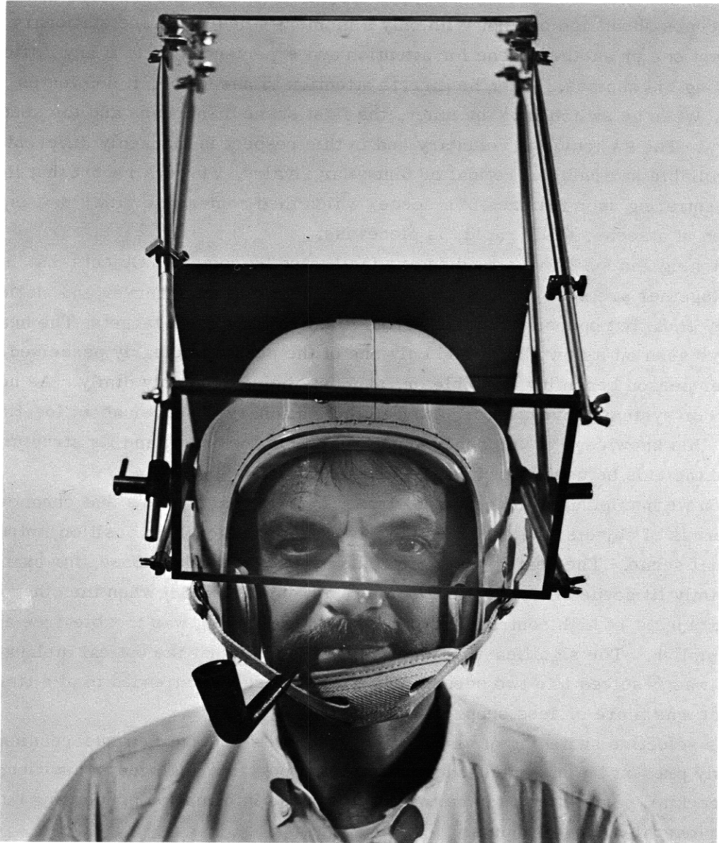
Fig. XXVI-2. Front view of the device. The half-silvered mirror is in place before the observer's eyes.
