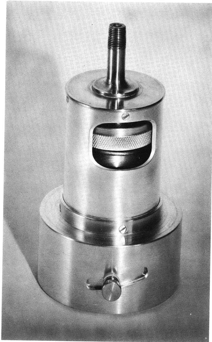
Fig. XVIII-3. The vacuum cutoff switch.
