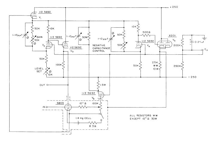
Fig. XVI-1. Electronic electrometer circuit.
