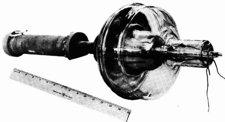
Fig. VIII-1 High voltage cathode ray tube
