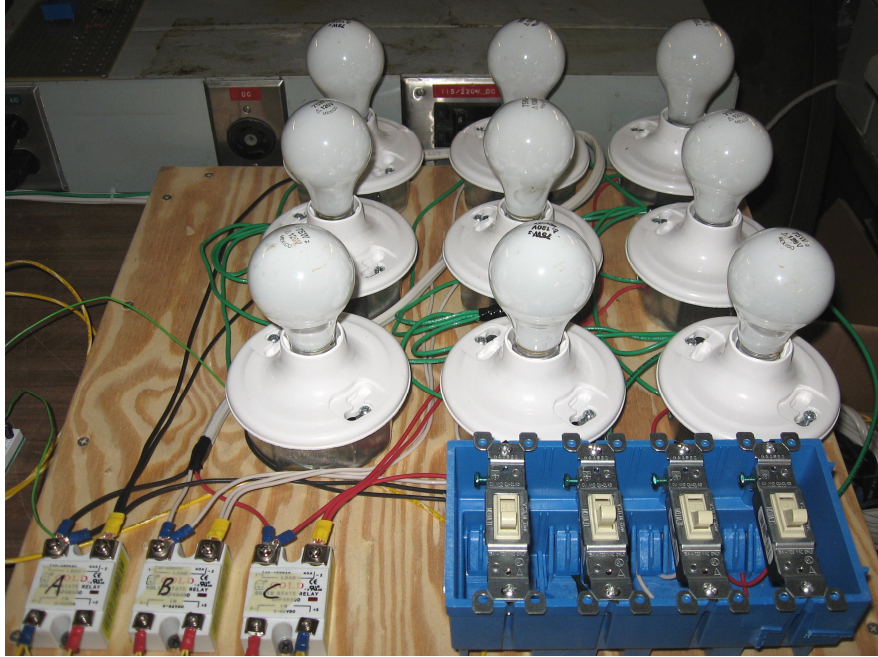
Figure 32: Loading Scheme for Response Testing
