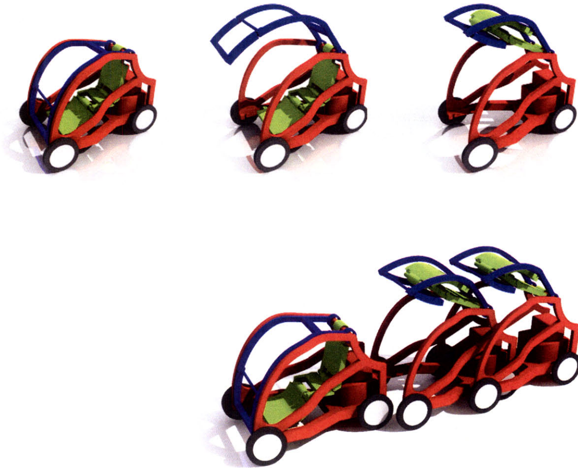
Fig 6.3 (above) Folding and stacking sequence for a collapsible car by Franco Vairani and Will Lark Jr.
