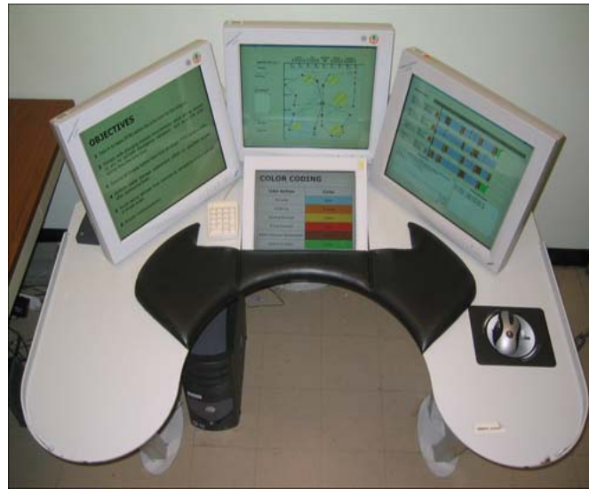
Figure 14: The Multi-Modal Workstation (MMWS)
