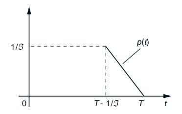
• For  $t = T - 1/\gamma$ , p(t) is equal to  $1/\gamma$ , so  $u^*(t)$  changes to  $u^*(t) = 1$ .
