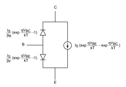
Complete model has only three parameters:  $I_S$ ,  $\beta_F$ , and  $\beta_R$ .
