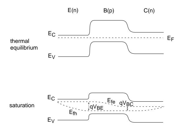
In saturation, collector and base flooded with excess minority carriers  $\Rightarrow$  takes lots of time to get transistor out of saturation.
