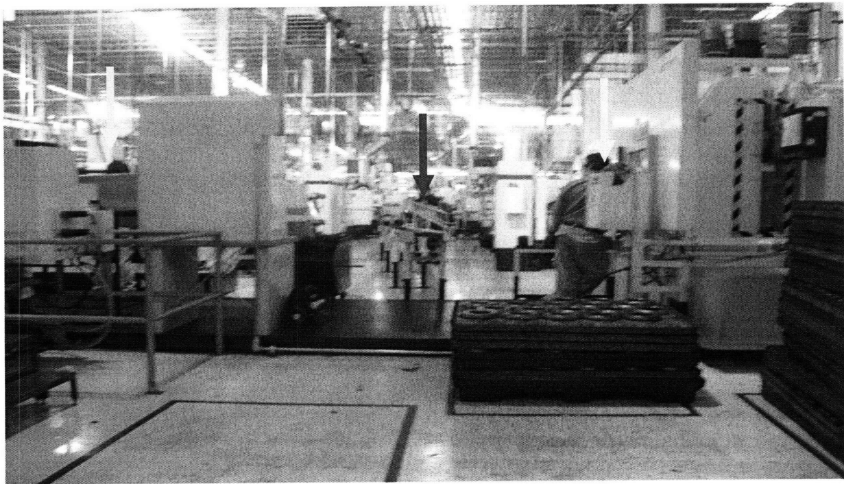
Figure 7: Operator Station in Guanajuato Factory (Operator picks part from machine near yellow arrow. The operator is supposed to place part on conveyor for next operation near red arrow.)
