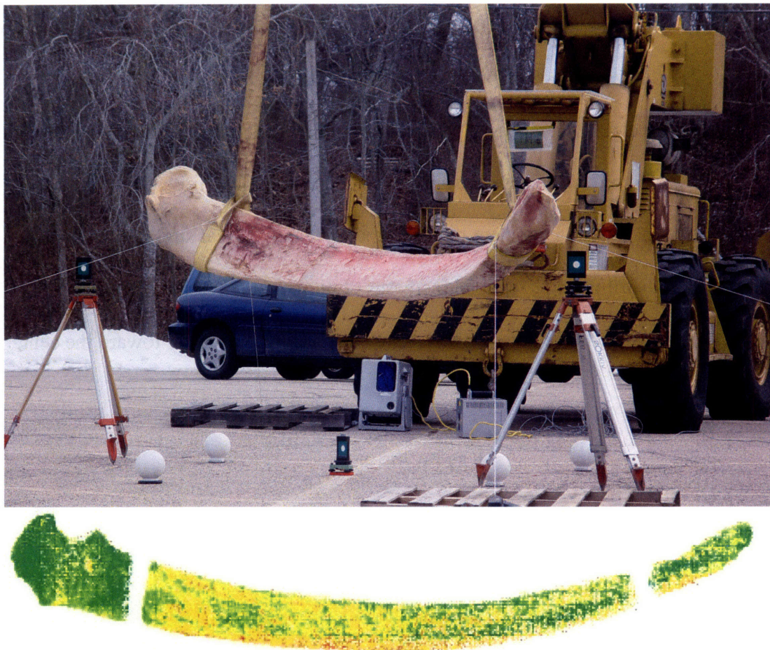
Figure 5.1: Three-dimensional laser scan of right whale mandible produces CAD-compatible point cloud detailing the external geometry of the bone. a) Above, the bone was strung from a crane such that it was free to be scanned in its entirety. b) Below, the resulting point cloud image that was transformed into a finite element mesh. In both images, the caudal end is at left, while the rostral apex is at the right. The image gaps in b designate the location of holding straps visible in a.
