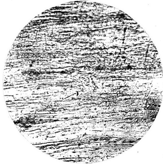
(7) A_{10} .10% C., Annealed at 1600° F After passing through 10th. draft longitudinal section 500 X
